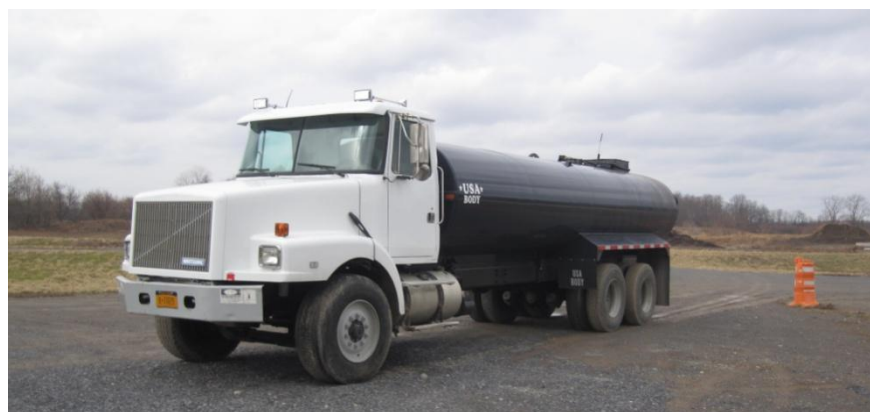
Figure 2. 4,500 Gallon tanker truck used for hauling manure to site and digested effluent from site
