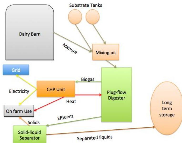
Figure 2. Lamb Farms digester flow diagram
