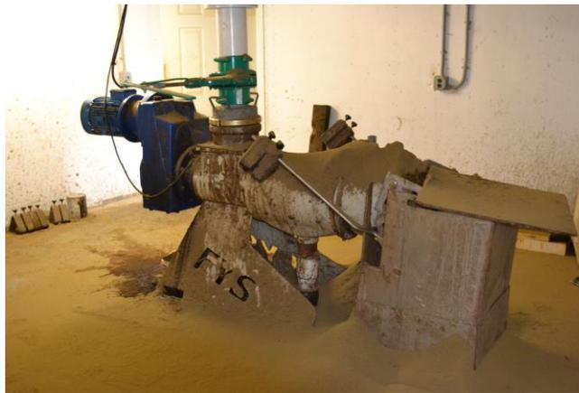
**Figure 3. Solid-liquid separator**
