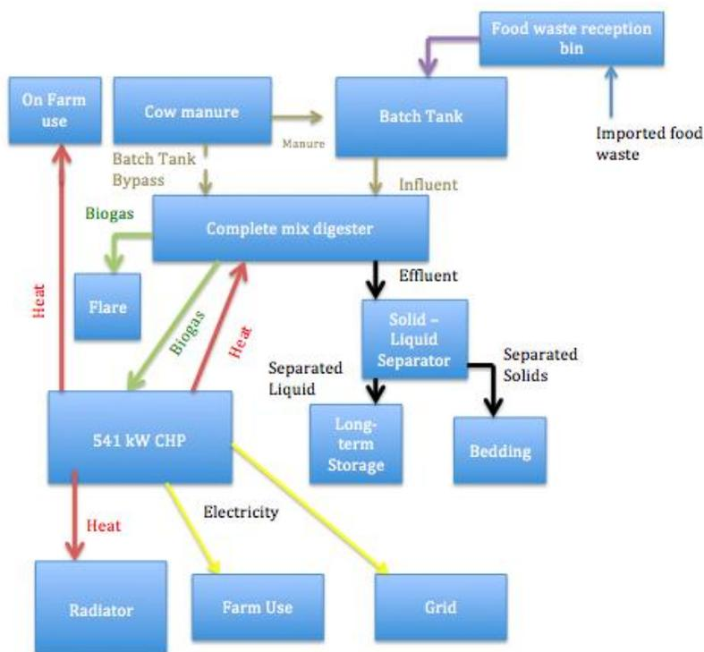
**Figure 1. Lawnhurst Farm AD system flow diagram**
