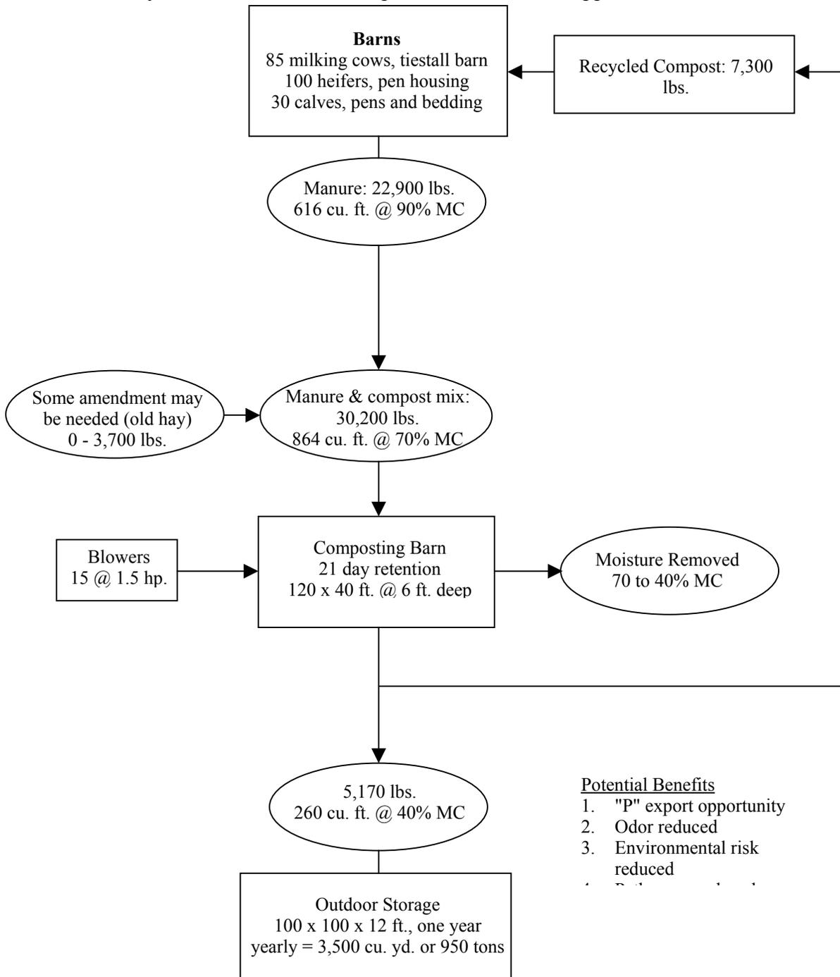
**Figure 4. Schematic of biodrying system on a farm showing daily amounts.**
