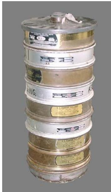
**Figure 1. Screens used to perform a sand particle size distribution analysis (sieve analysis).**
