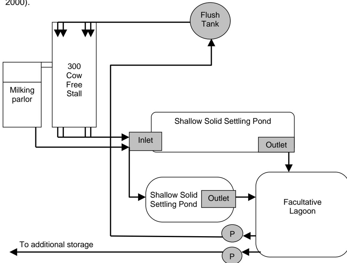
Figure 5. Bion system schematic.
