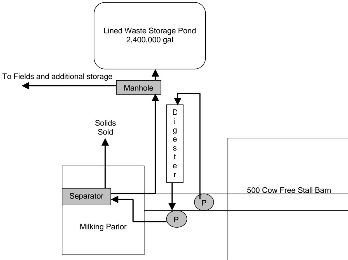
Figure 3. Anaerobic digester schematic for a 500 cow dairy farm.
