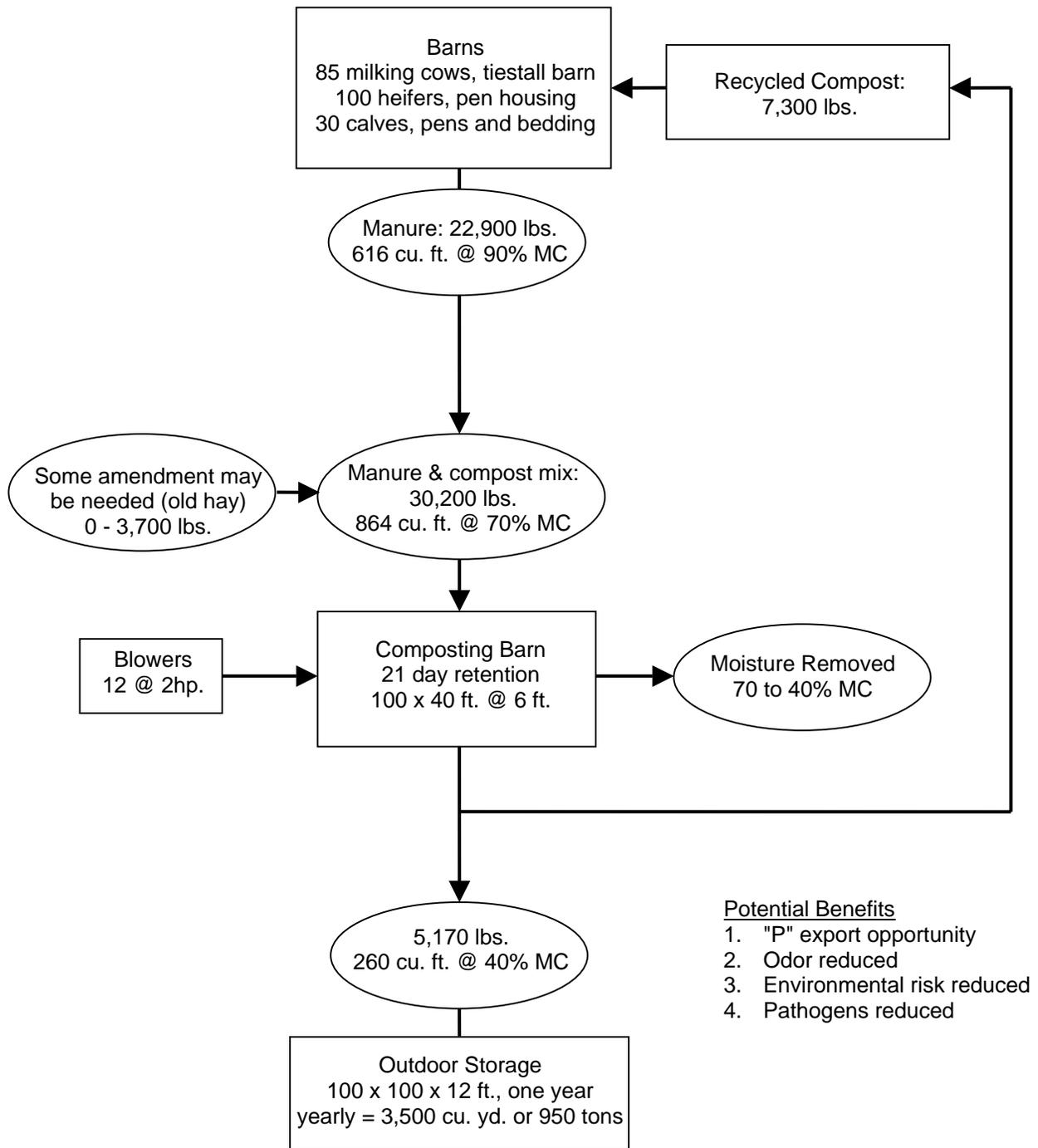
Figure 2. Biodrying schematic for 133 cow equivalents.
