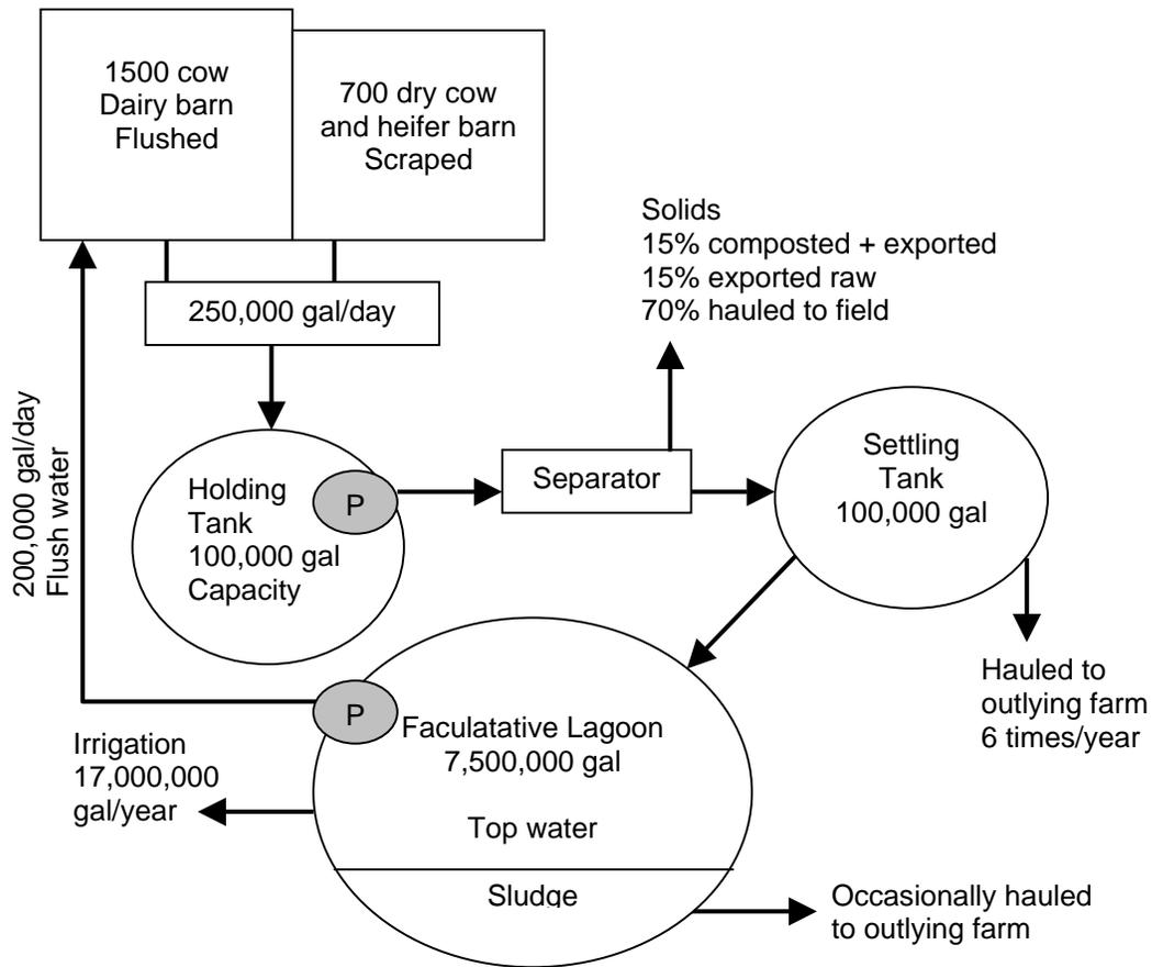
Figure 6. NC system schematic for a 1980 cow equivalents.
