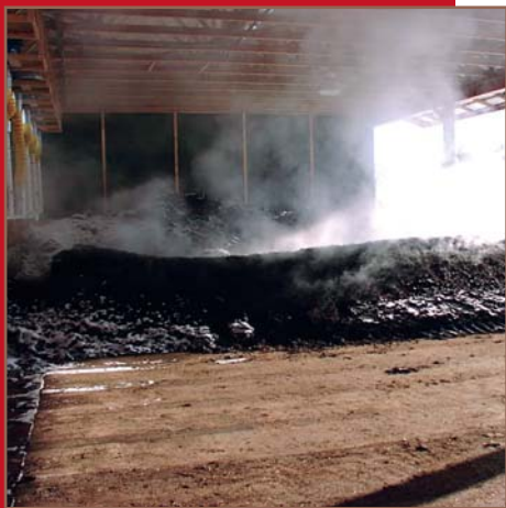
Compost while being aerated inside biodrying building
