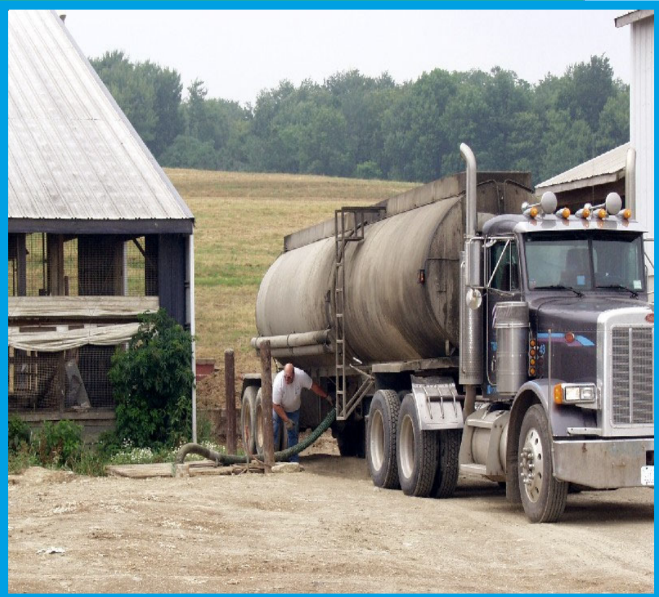
Addition of Food Waste to Reception Pit of an Anaerobic Digester at Matlink Dairy Farm.
