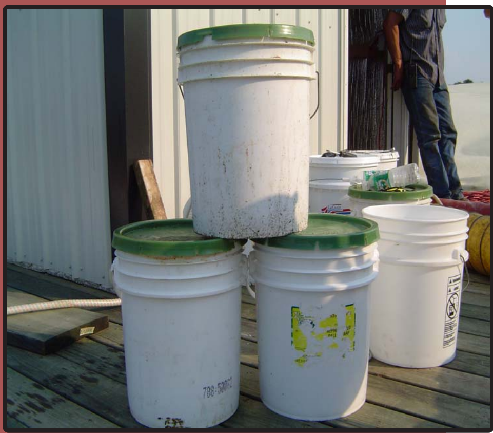
Used restaurant grease, added to the influent pit weekly with the goal of reducing foaming
