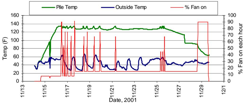
**Figure 2-3. Composting Run with Heifer Manure, Resulting in Inadequate Air for Moisture Removal, Bay 5.**
