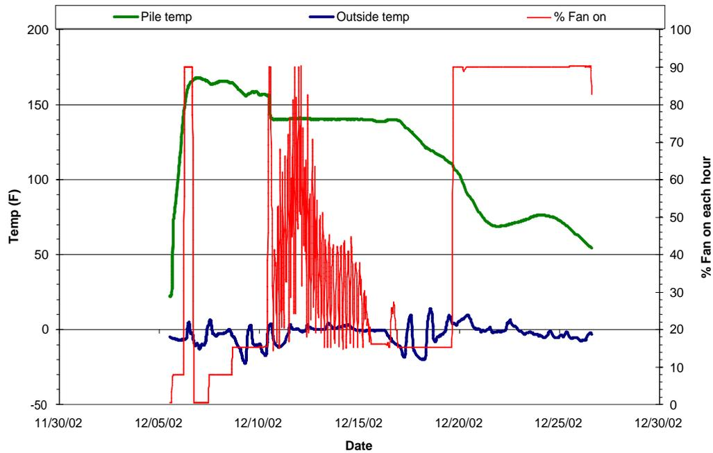
**Figure 2-7: The Pile Temperature and Percent per Hour the Fan Ran for Bay 5 in Negative Pressure.**
