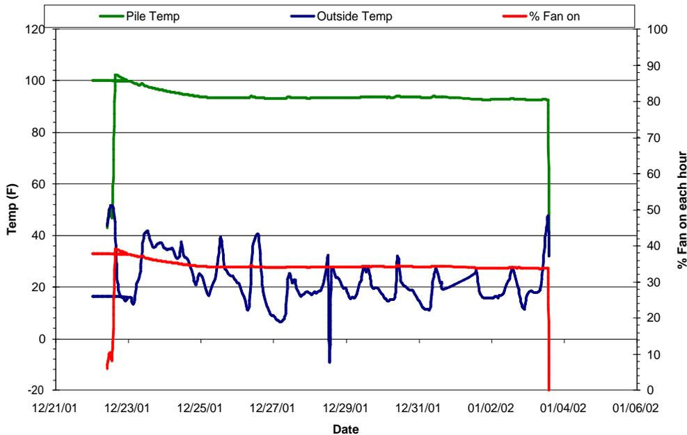
**Figure 2-5. Low Heat Composting Run with Minimum Fan On-Time in Cold Weather, Bay 8.**
