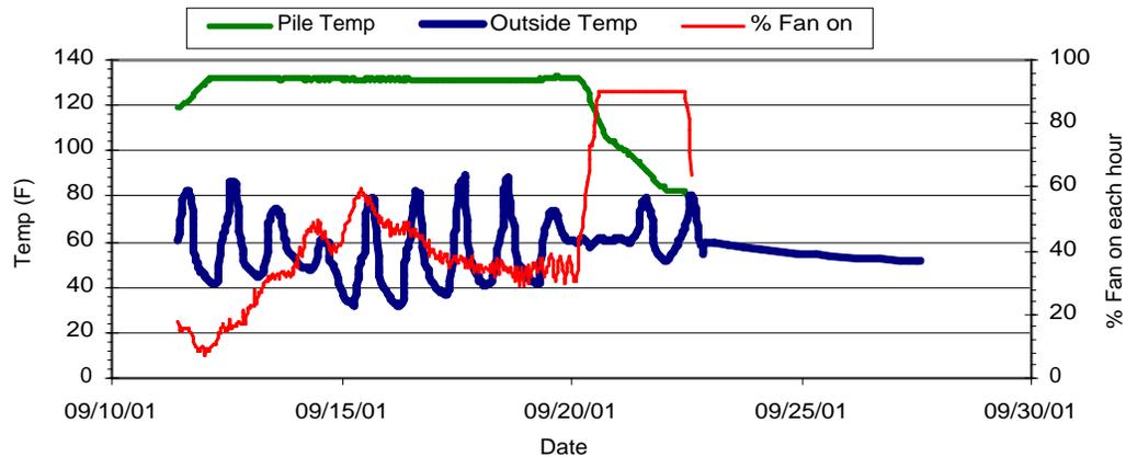
**Figure 2-1. Successful Composting Run with Good Fan Control and Drying, Bay 1.**
