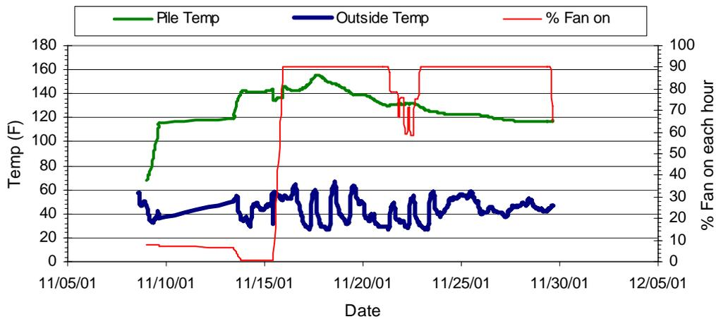
**Figure 2-2. Unsuccessful Composting Run with Inadequate Air Delivery, Bay 1.**
