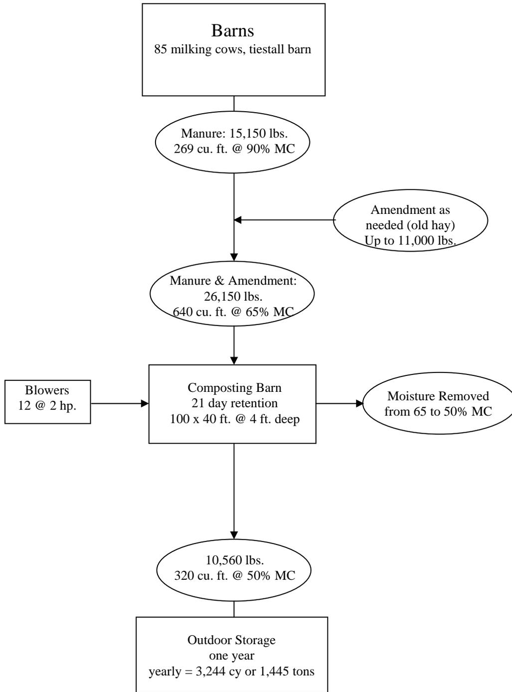
**Figure A-1. Schematic of Biodrying System on a Farm Showing Estimated Daily Amounts.**
