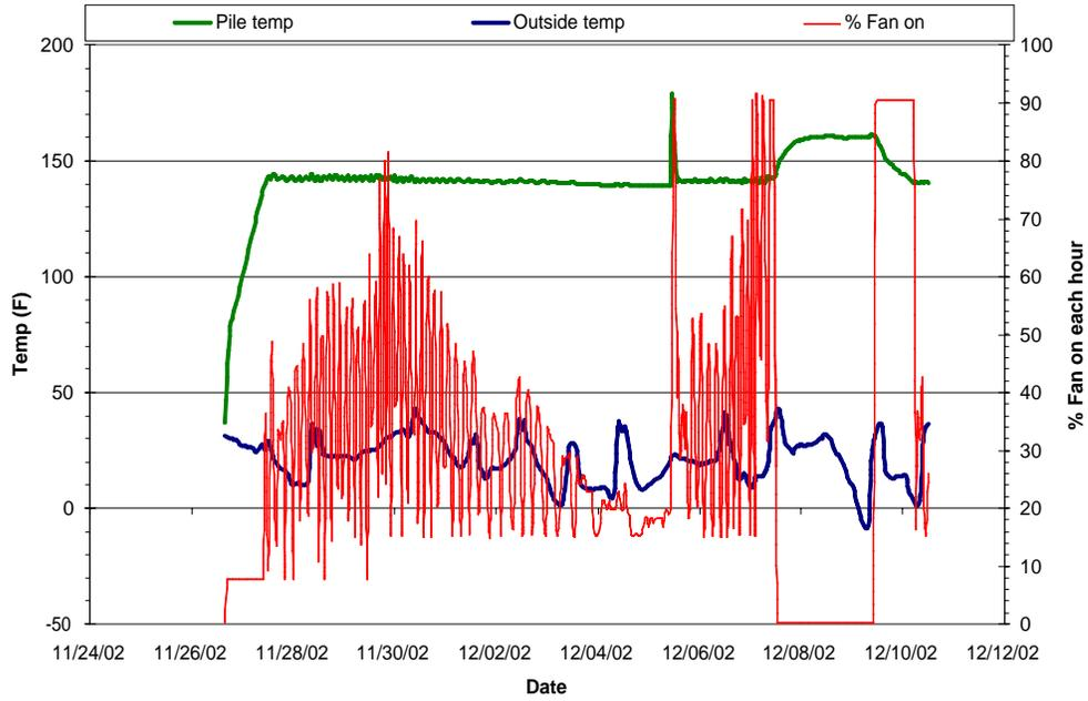
**Figure 2-6: The Pile Temperature and Percent per Hour the Fan Ran for Bay 1 in Negative Pressure.**
