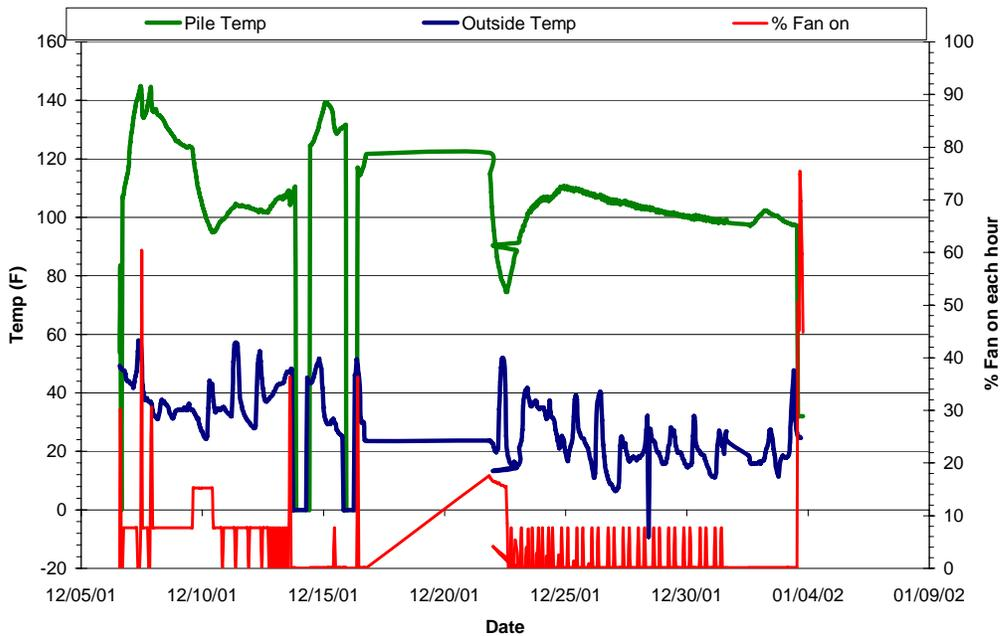
**Figure 2-4. Composting Run with Over Aeration in Cold Weather, Bay 6.**
