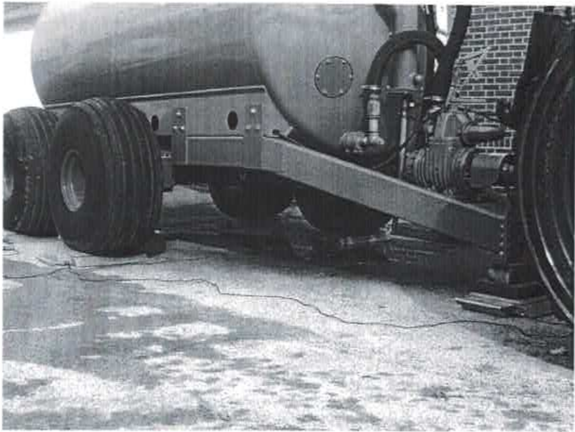
Figure 1. Vacuum loaded slurry tank used for flow v. pressure testing.
