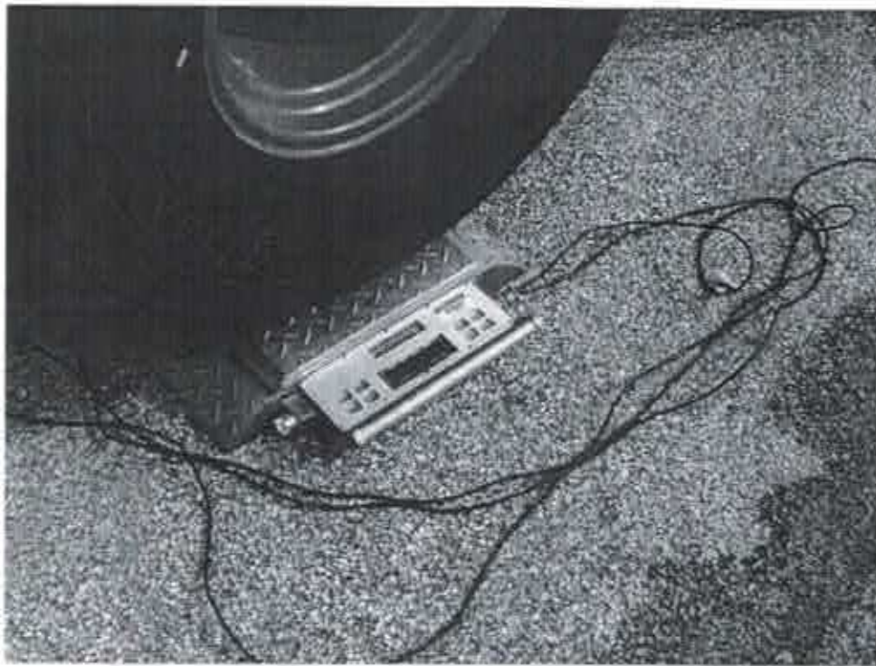
Figure 5. One of five interconnected wheel scales used for monitoring slurry tank weight during flow tests.
